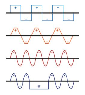
**AC Square Wave:** Allows the current to change from electrode (+ positive) to electrode (- negative) very quickly. This produces high voltage as the current switches polarities allowing the arc to restart easily. The arc can be maintained without the use of high-frequency and the fast transitions provide for responsive, dynamic and focused arc for better directional control.
